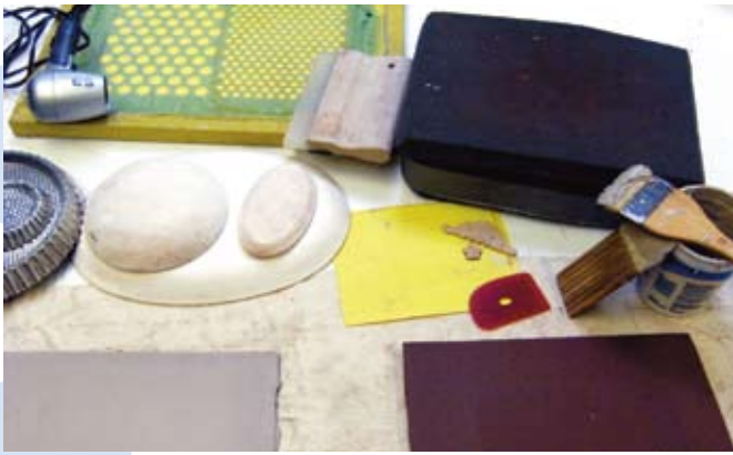
Tools and supplies for this process include simple hump/drape molds and 3-inch blocks of soft foam. Texturing tools, cutters and printing supplies are all optional.
